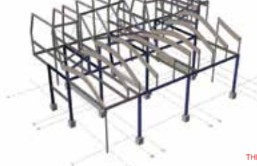
BRACED FRAME THIRD FLOOR
