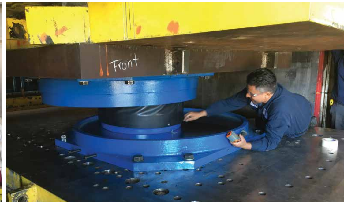
▲ TRIPLE PENDULUM ISOLATOR TESTING, DISPLACEMENT
